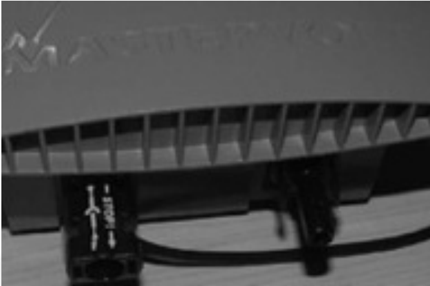
Figure 3-4: Mastervolt Soladin 600 Inverter with one pair of MC Type 4 connectors
