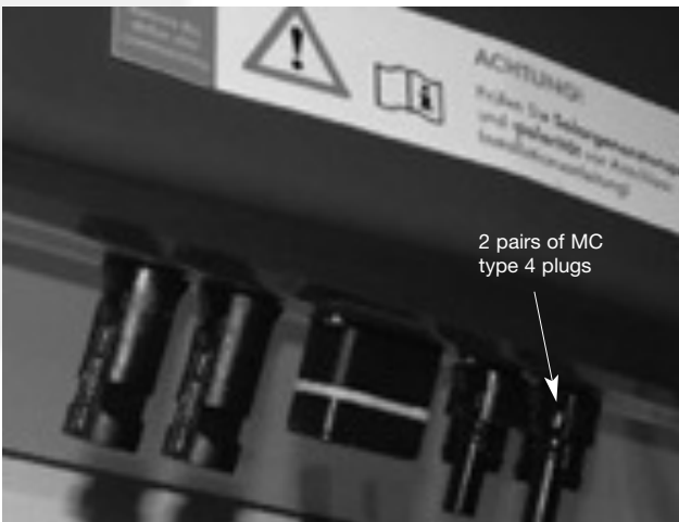
Figure 3-6: SMA Sunny Boy Inverter with two pairs of MC Type 4 connectors
